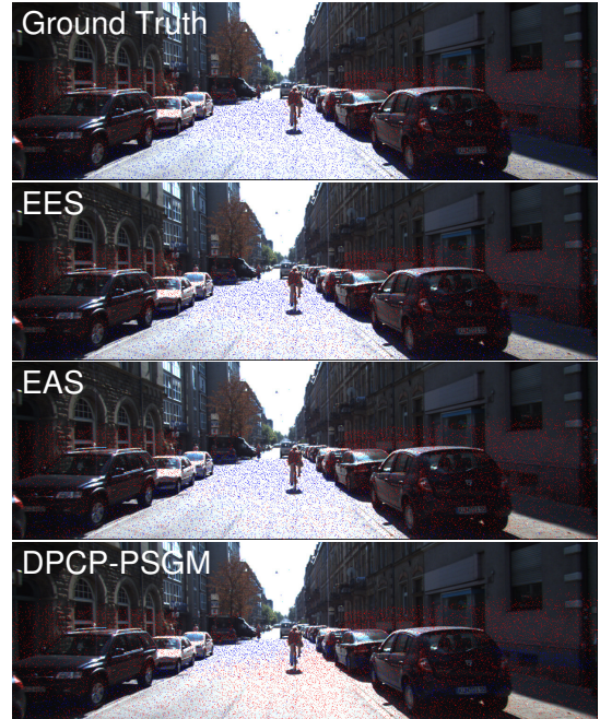
Fig. 3: Frame 153 of dataset KITTI-CITY-5: an illustrative example of 3D point cloud road plane fitting, raw image, projection of annotated 3D point cloud onto the image, and detected inliers/outliers using a ground-truth threshold on the distance to the hyperplane for each method. Blue indicates classified inlier points and red indicates the opposite. The noise level is 0.12, the outlier ratio is 0.67. The AUC value for EES, EAS and DPCP-PSGM are 0.971, 0.932 and 0.757.
